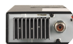
Large size heatsink provides heat dissipation for the high power Mosfet RD16HHF1
